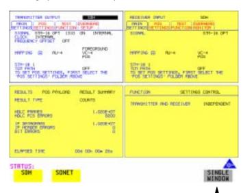
Press this key to select single window mode. The active window is then displayed (in this example - TRANSMITTER OUTPUT would be displayed).
