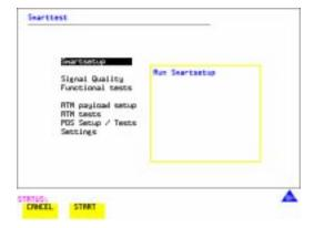
With Smartsetup highlighted, press **START** to auto-discover information about the receive signal. Or press **CANCEL** to exit Smart Tests.
